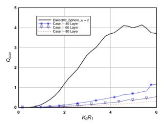
Figure 6. The normalized total scattering cross section for cloaked dielectric sphere with  $\varepsilon_d = 2$  for different numbers of layers, case I,  $c = R_1/40$ .
