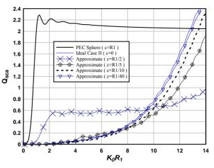
Figure 3. The normalized total scattering cross section of cloaked conducting sphere for different values of c (40-Layers) [21].
