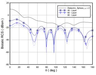
Figure 13. Bistatic RCS for different numbers of layers for case II ( $\varepsilon_d = 2$ ) at  $c = R_1/40$ .
