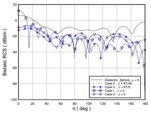
Figure 9. Bistatic RCS of cloaked dielectric sphere with  $\varepsilon_d = 5$  for different values of c, 2M = 40.
