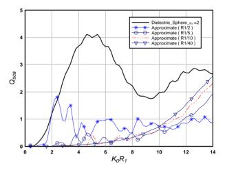
Figure 4. The normalized total scattering cross section of cloaked dielectric sphere  $\varepsilon_d = 2$ , with multi-layered isotropic structure for different values of *c*, case II, 2M = 40.
