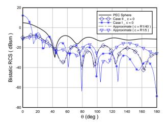
Figure 10. Bistatic RCS of cloaked conducting sphere for different values of c, 2M = 40 [21].
