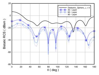
Figure 14. Bistatic RCS for different numbers of layers for case II ( $\varepsilon_d = 5$ ) at  $c = R_1/40$ .
