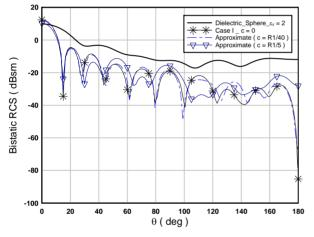
Figure 11. Bistatic RCS of cloaked dielectric sphere for different values of c for case I at  $\varepsilon_d = 2$ , 2M = 40.
