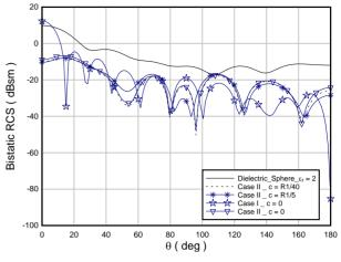
Figure 8. Bistatic RCS of cloaked dielectric sphere with  $\varepsilon_d = 2$  for different values of c, 2M = 40.
