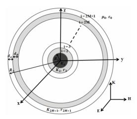
Figure 2. Plane wave scattering by a multi-layer dielectric sphere.
