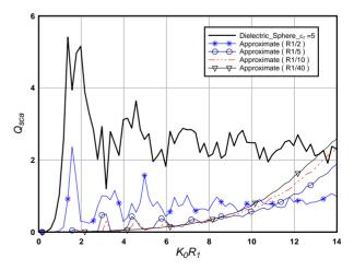
Figure 5. The normalized total scattering cross section of cloaked dielectric sphere  $\varepsilon_d = 5$ , for different values of *c*, case II, 2M = 40.
