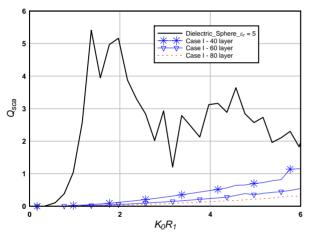
Figure 7. The normalized total scattering cross section for cloaked dielectric sphere with  $\varepsilon_d = 5$  for different numbers of layers, case I,  $c = R_1/40$ .
