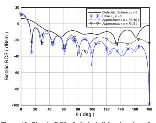
Figure 12. Bistatic RCS of cloaked dielectric sphere for different values of c for case I at  $\varepsilon_d = 5$ .
