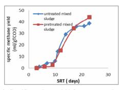
Figure 2. Specific methane yield from untreated and pretreated mixed sludge.
