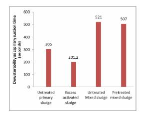
Figure 4. Dewaterability of different sludge samples.
