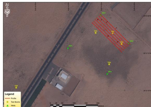
Figure 5. Satellite image showing the location of the 2D electrical resistivity profiles and borehole locations.
