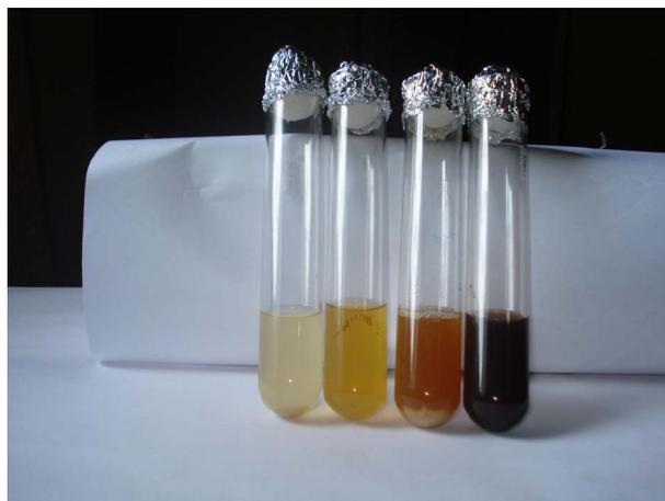
**Figure 2. Photograph of change in colour of aliquot after addition of AgNO<sub>3</sub> during different time period (from left to right): control, 24 hrs, 48 hrs and 72 hrs.**
