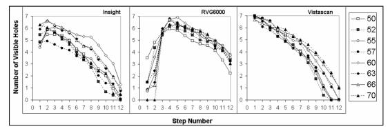
**Figure 6.** The variation of the average number of visible holes in each one of the 12 steps (considering only the images with the highest TS for each tube current setting) is given for the different tube potential settings used.
