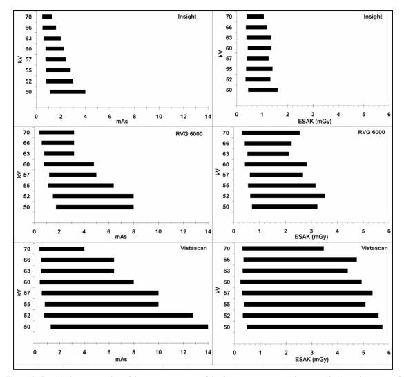
**Figure 3.** Graphical representation of the exposure ranges of the three receptors tested in terms of mAs and in terms of ESAK used to obtain the stepwedge phantom images at all tube potential settings.
