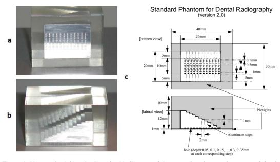
Figure 1. Photographs (a,b) and schematic; (c) diagrams of the stepwedge phantom that was used for the evaluation of image quality.
