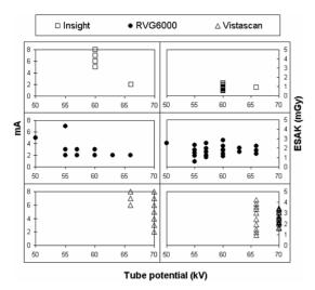
**Figure 5.** The distribution of images with TS larger or equal with the 90% of the largest total score observed for each receptor overall, with respect to the mA setting and the ESAK at all tube potential settings is shown.
