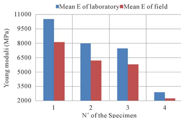
Figure 7. Graphical representation of Young moduli for different kinds of specimens of sandstones (1: white sandstones; 2: red sandstones; 3: purple sandstones; 4: sandstones with intercalation of pelites).
