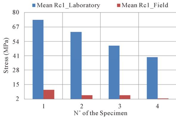
**Figure 8. Graphical representation of uni-axial compression stress for different kinds of specimens of sandstones (1: white sandstones; 2: red sandstones; 3: purple sandstones; 4: sandstones with intercalation of pelites).**
