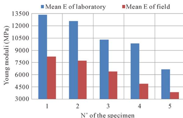
Figure 6. Graphical representation of Young moduli for different kind of basalts in laboratory samples and field ones (1: healthy basalts, 2: basalts with unfilled fractures, 3: basalts with tension cracks filled with quartz, 4: basalts with multiple fractures, 5: basalts with fractures filled with calcite, chlorite, epidote).
