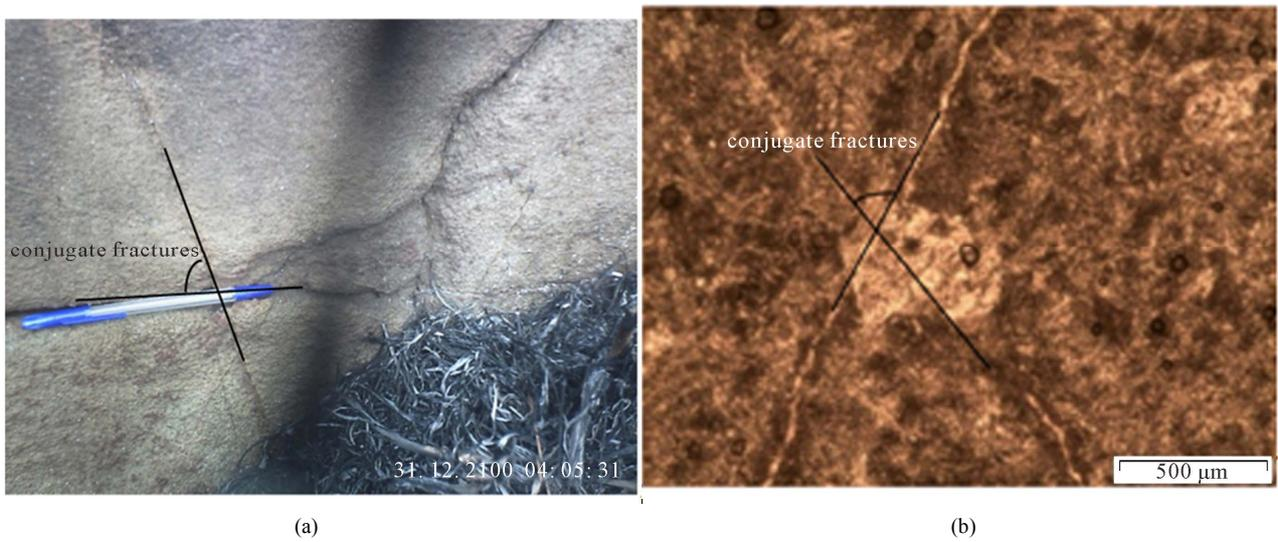
Figure 10. Fractal geometry in conjugate fractures ((a) outcrops scale; (b) preparation scale).
