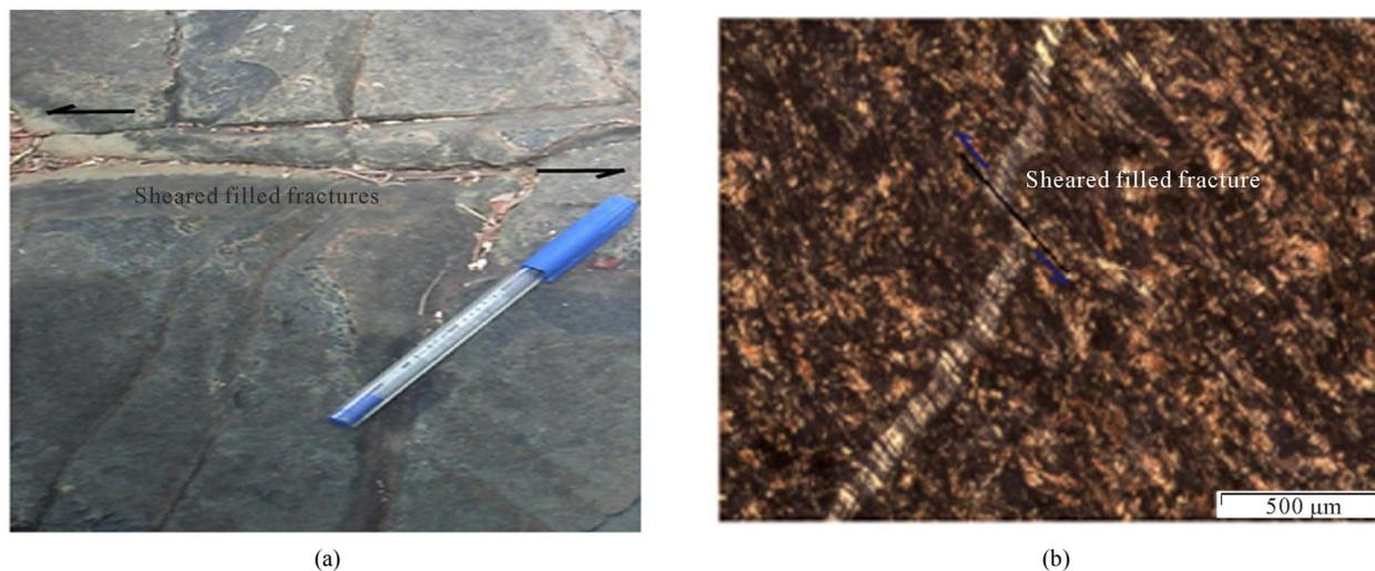
Figure 11. Microscopic shear of filled microdiscontinuity ((a) outcrops scale; (b) preparation scale).
