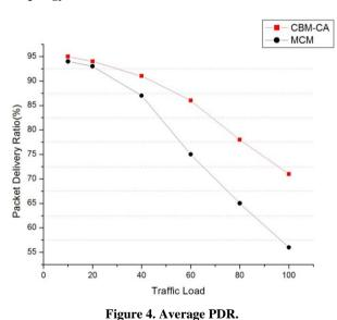
of packet send and no. of packet receive is high means no. of packet deliver at each link. In the figure we see when traffic load is 10 packet/s then the packet delivery ratio for CBM-CA schemes near about 90% and when the traffic load is 100 packet/s the PDR is above 70% that is good in comparison to MCM.
