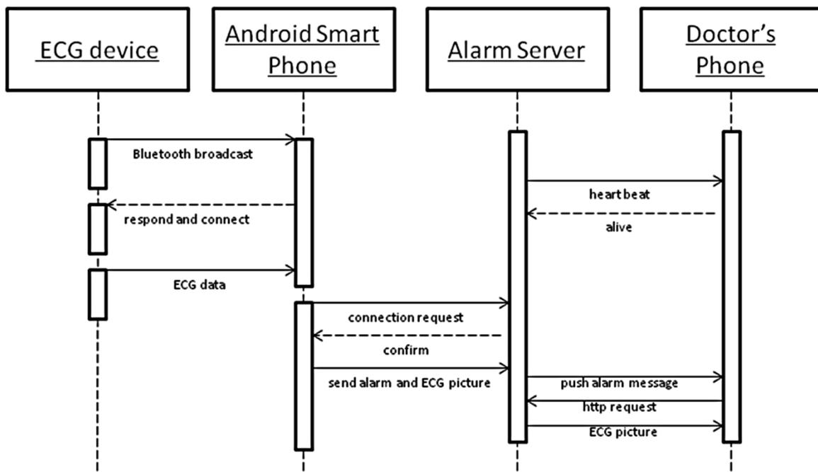
**Figure 4.** Process of an alarm in the system.
