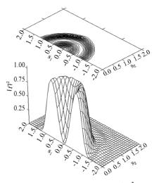
Figure 13. The synthesized power DP  $|f|^2$  of the plane aperture for prescribed DP (29).
