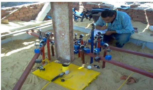
**Figure 3.** Settlement readings at surface using dial gauges.
