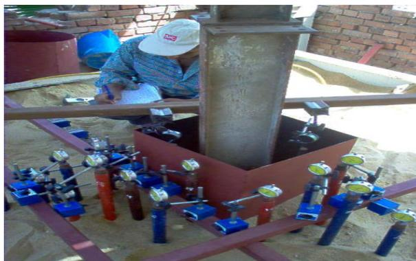
**Figure 5.** Settlement readings in case of surcharge using square steel box.
