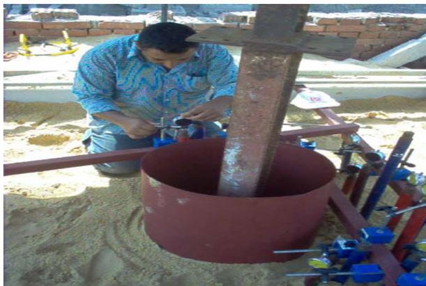
**Figure 4.** Settlement readings in case of surcharge using circular steel box.
