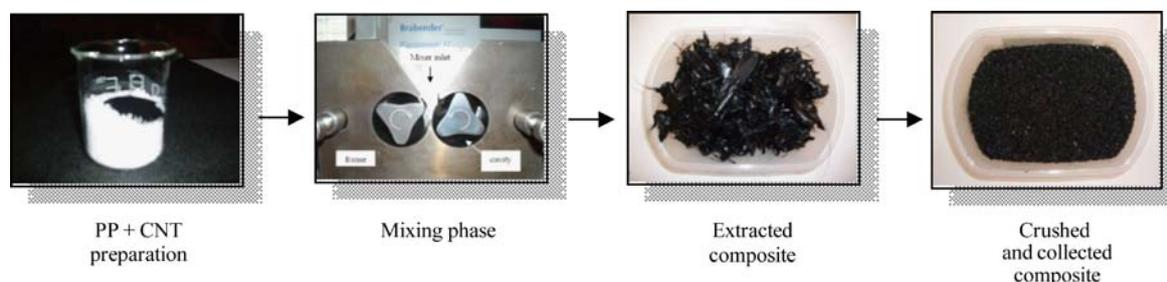
**Figure 1.** Manufacturing phase of the PP/MWCNT composite.
