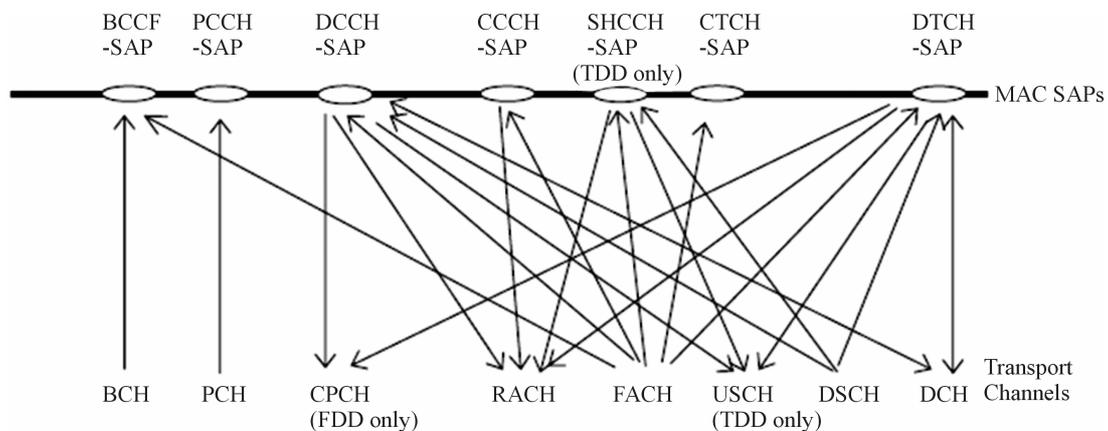
**Figure 5. Logical channels mapped onto transport channels, seen from the UE side [8].**
