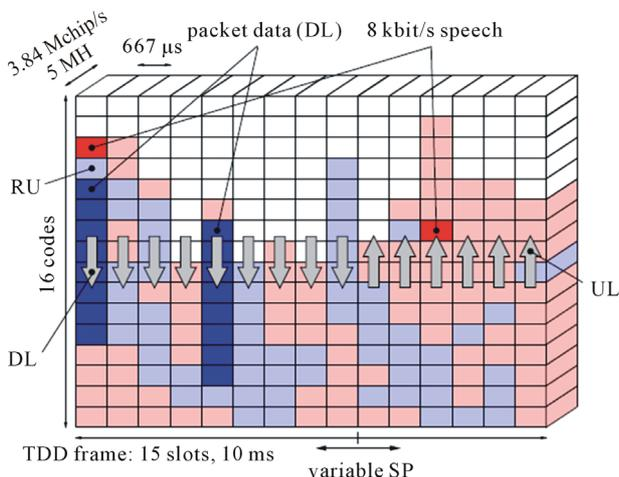
**Figure 6. Radio frame configuration in UTRA-TDD with asymmetric time slot [12,13].**
