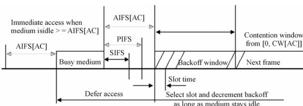
**Figure 1. The channel access scheme for IEEE 802.11e EDCA [5].**
