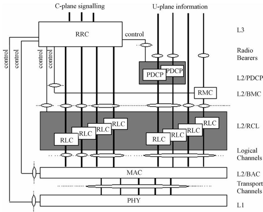
**Figure 4. Radio interface protocol architecture. The service access points are marked by circles [7,8].**
