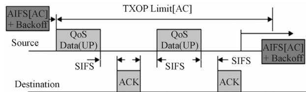
**Figure 2. The temporal working structure of EDCA TXOP [5].**
