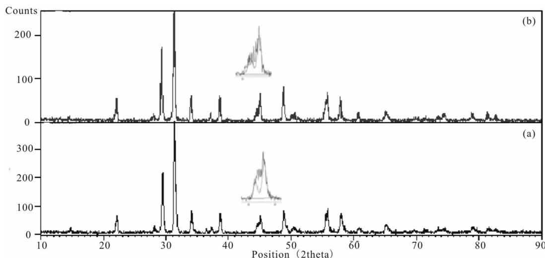
**Figure 1.** XRD patterns of PZS-PLZT ceramics sintered at (a) 1050°C and (b) 1200°C.
