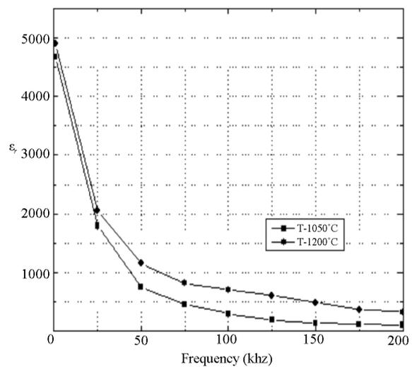
Figure 4. Frequency dependence of  $\epsilon_r$  for PZS-PLZT samples sintered at 1050°C and 1200°C.
