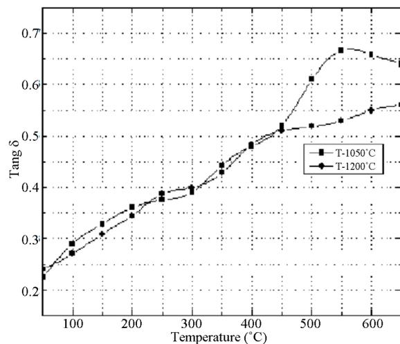
Figure 5. Temperature dependence of  $\text{Tang } \delta$  for PZS-PLZT samples sintered at 1050°C and 1200°C.
