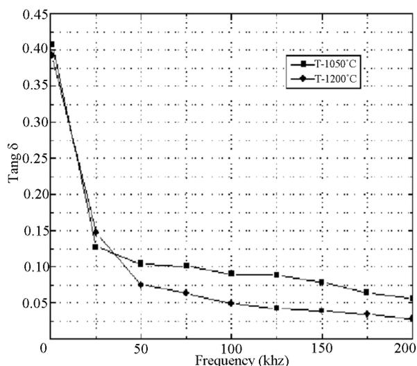
**Figure 6.** Frequency dependence of  $Tang\delta$  for PZS-PLZT samples sintered at 1050°C and 1200°C.
