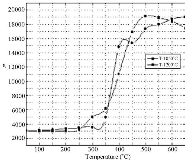
Figure 3. Temperature dependence of  $\epsilon_r$  for PZS-PLZT samples sintered at 1050°C and 1200°C.
