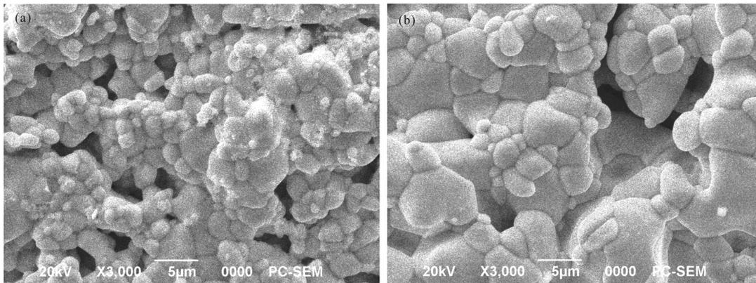
Figure 2. SEM micrographs of PZS-PLZT ceramics sintered at (a) 1050°C; (b) 1200°C for 2 hours.
