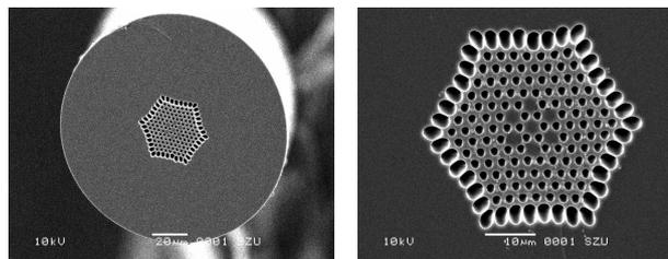
**Figure 1. SEM pictures of seven-core PCF: (a) the end face (b) the core region.**
