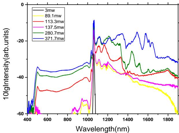
**Figure 6. Spectral evolution of seven-core PCF for different output power.**
