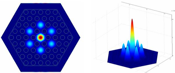
Figure 2. Calculated mode profiles of supermodes in seven-core PCF.
