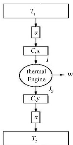
**Figure 1.** Thermal engine working between both  $x$  and  $y$  temperatures. The reservoirs are at temperatures  $T_1$  and  $T_2$ . The fluxes to the engine and from the engine are respectively  $J_1$  and  $J_2$ .
