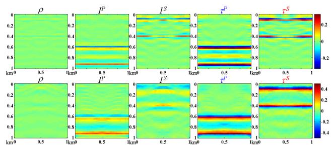
Figure 6. R-solutions for the model shown in Figure 2. In the upper layer - perturbation of S-wave attenuation, in the lower – of P-wave attenuation. In the first line of the condition number is 100 and the frequency range (5.30) Hz in the second - the condition number is 1000 and a frequency range is (5.45) Hz.
