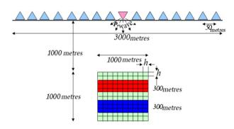
Figure 2. Mathematical model of the medium. Target area is a square. The red part has perturbation of the S-wave impedance, in blue – P-wave impedance; second case: S-wave attenuation - in red and P-wave attenuation - in blue.
