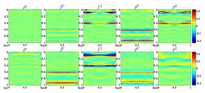
Figure 5. R-solutions for the model shown in Figure 2. In the upper layer - perturbation of S-wave impedance, in the lower – of P-wave impedance. In the first line of the condition number is 100 and the frequency range (5.30) Hz in the second - the condition number is 1000 and a frequency range is (5.45) Hz.
