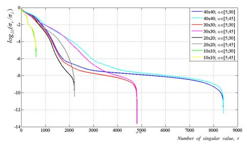
Figure 3. Singular values in the logarithmic scale for different grids(in metres) and frequency ranges (in Hz).
