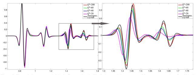
Figure 7. The scaled trace recorded in the first receiver in Fig. 2. Assumed the presence of P-wave attenuation: Q = 200, 60, 40, 20, and also in the linearized case. Right picture is zoomed rectangle from the left picture.
