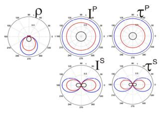
Figure 1. Diffraction patterns for the incident P-wave for frequencies 25 Hz, 15 Hz, 10 Hz (blue, red, black colors).
