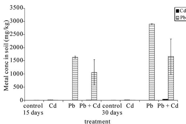
**Figure 1. Cadmium and lead concentrations in soil microcosms (mg/kg).**
