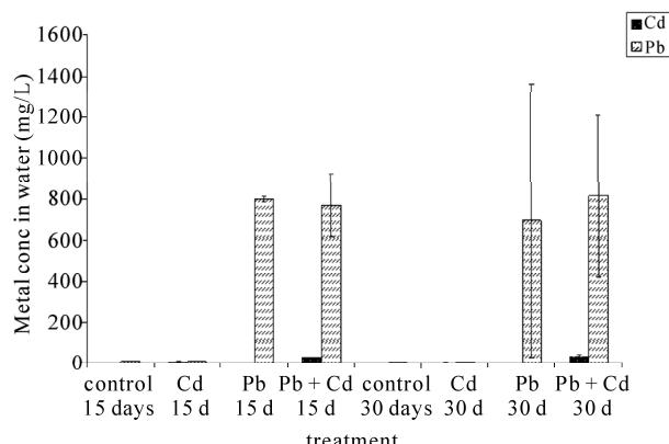
**Figure 2. Cadmium and lead concentrations in water microcosm (mg/L).**
