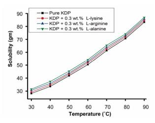
Figure 2. Solubility curves for pure and 0.3 wt% L-arginine, L-lysine, L-alanine doped KDP crystals.
