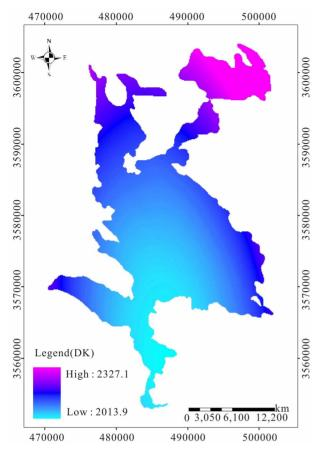
Figure 7. Grounwater levels map in Shahrekord plain using DK model.
