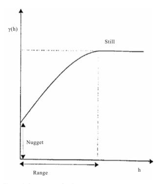
Figure 4. Components of variogram.
