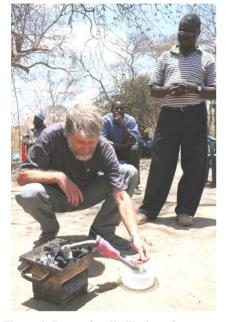
Figure 2. Retort for distillation of mercury.
