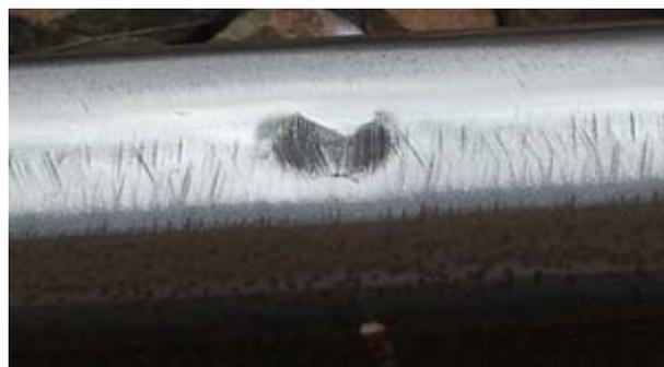
**Figure 1.** Squat defect on the running surface or ball of the rail head.
