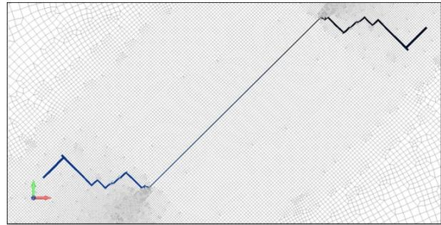
**Figure 6.** The crack growth result of the validation model.
