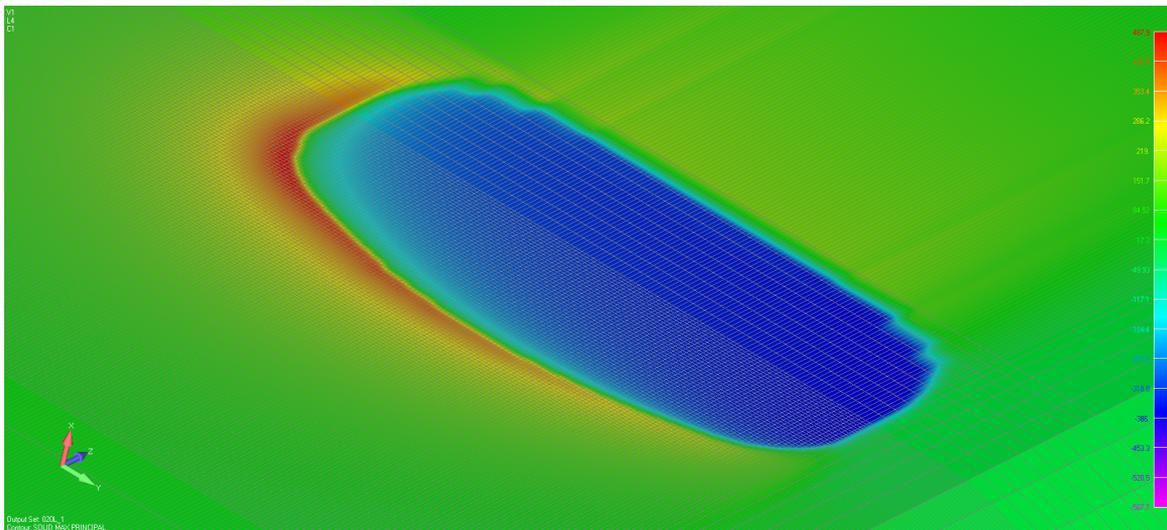
Figure 13. Maximum principle stress of the rail under contact loads at initial time.
