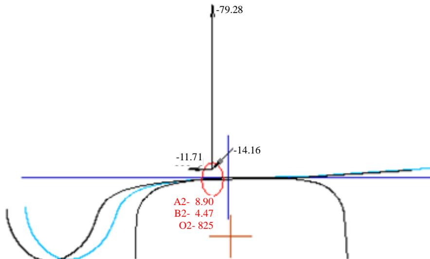
Figure 9. Contact forces at low rail [7].
