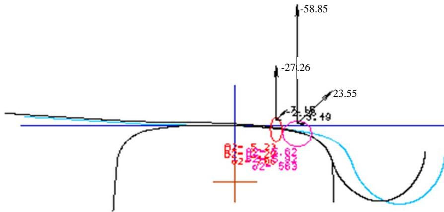
Figure 10. Contact forces at high rail [7].
