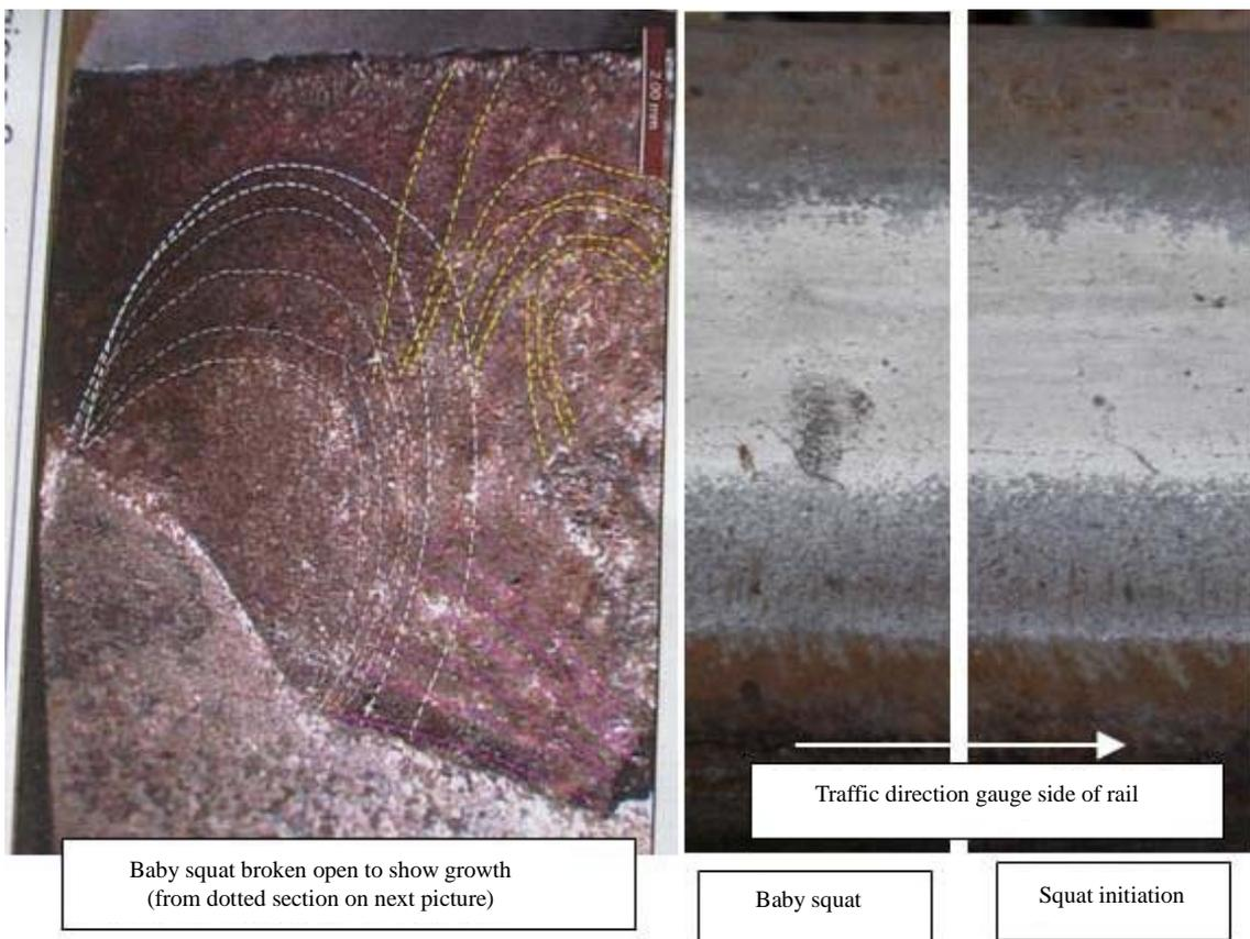
Figure 3. The initial squat growth appears to arise from a similar crack position and orientation.
