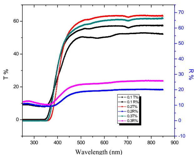
**Figure 3.** The transmittance T% and the Reflectance R% of unirradiated LTbPTiO<sub>2</sub> with different concentration of TiO<sub>2</sub>.
