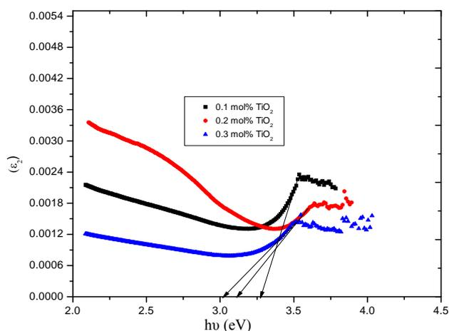
Figure 7. The relation between Optical dielectric constant  $\epsilon_2$  and phonon energy for irradiated LTBPTiO<sub>2</sub> system.
