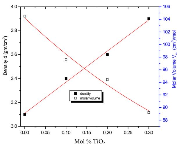
**Figure 1.** Variation of density and molar volume with TiO<sub>2</sub>% unirradiated for the glass system LTbPTiO<sub>2</sub>.
