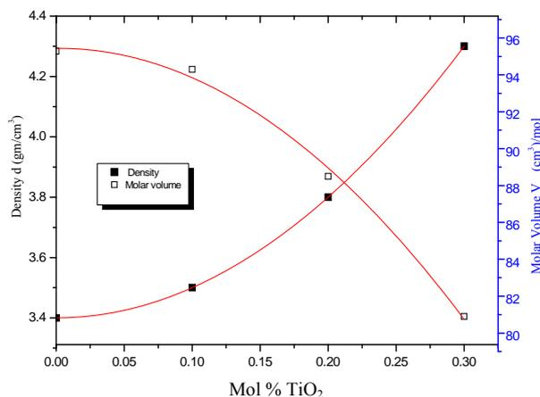
**Figure 2.** Variation of density and molar volume with TiO<sub>2</sub>% irradiated with 3 Mrad gamma dose for the glass system LTbPTiO<sub>2</sub>.
