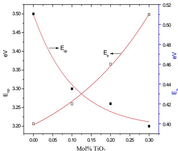
Figure 8. Variation of optical band gap  $E_{op}$  and band tail  $E_e$  with TiO<sub>2</sub> mol% for unirradiated glass system LTBPTiO<sub>2</sub>.
