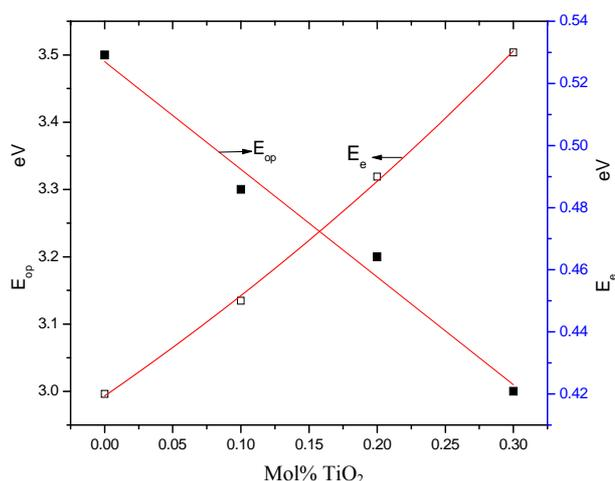
Figure 9. Variation of optical band gap  $E_{op}$  and band tail  $E_e$  with TiO<sub>2</sub> mol% for 3 Mrad gamma irradiation for the glass system LTBPTiO<sub>2</sub>.
