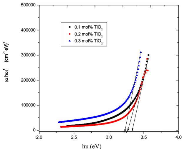
**Figure 6. The relation between energy  $h\nu$  eV and  $(\alpha E)^2$  for unirradiated glass ( $R$ : is the reability of fitting, best fitting  $R = \pm 1$ ).**
