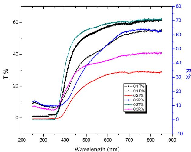
**Figure 4.** The transmittance T% and the Reflectance R% of 3 Mrad gamma irradiated LTbPTiO<sub>2</sub> with different concentration of TiO<sub>2</sub>.
