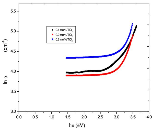
**Figure 5.** The relation between absorption coefficient  $\ln \alpha$  and energy  $h\nu$  for the prepared glass system.
