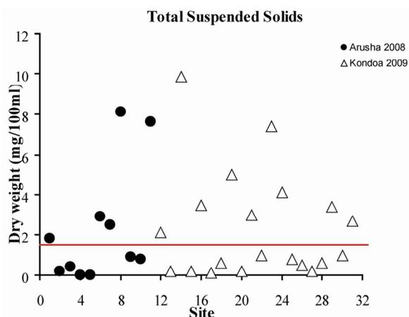
**Figure 3.** Total suspended solids for all sites, 2008-2009. The red line indicates the allowable limit of suspended solids for UV disinfection, 15 mg/L.
