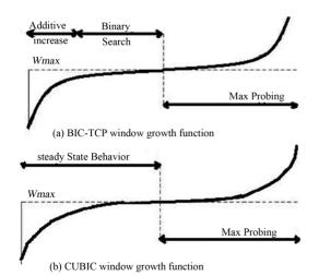
Figure 7. Window growth function for BIC-TCP and CU-
