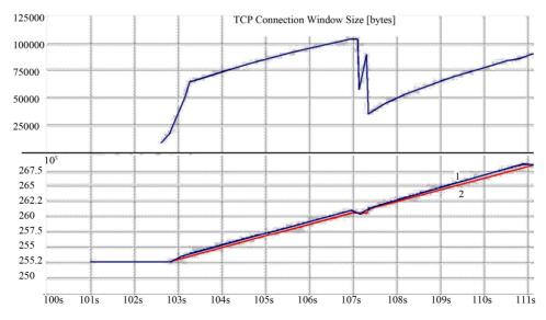
Figure 3. CWND changing (above) and the number of transmitted (line 1) and received segments (line 2) with time (below).
