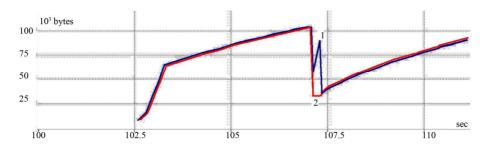
Figure 4. CWND changing for TCP Reno (line 1) and TCP SACK (line 2) when one segment loss.
