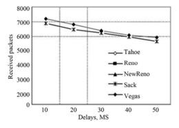
Figure 5. The number of received packets depending on packet delays.
