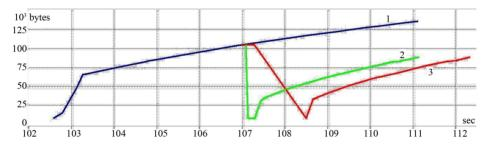
Figure 2. CWND changing: line 1—Tahoe when one segment loss; line 2—Tahoe when one segment loss; line 3—TCP Reno when one segment loss.
