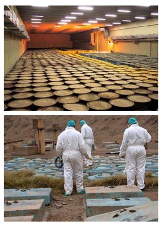
Figure 3. Left, waste barrels comprised of two groups, first; ready to use material (known as yellow cake), second; waste material stored in plastic barrels. Right, decayed solid and liquid radioactive wastes stored at Al-Tuwaitha site-waste silos (www.iaea.org).
