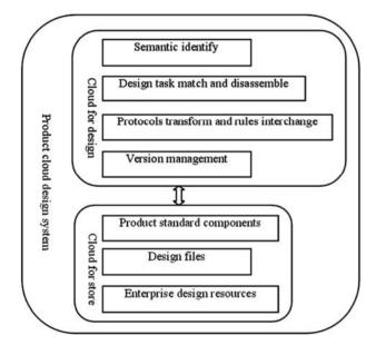
Figure 2. System functions of product cloud design.
