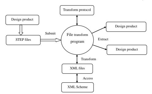
Figure 3. STEP & XML transform mode.
