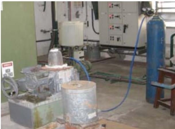
**Figure 1.** Alloy preparation setup consisting of induction furnace and argon cylinder.
