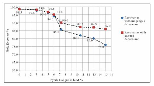
Figure 6. Curves showing gold recoveries before and after pyrite depression using lime at 90 minute contact time.
