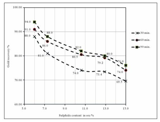
Figure 2. Gold recoveries from high sulphide ores with addition of surfactants.
