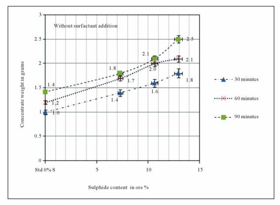
Figure 3. Concentrate weights attained due to gangue recovery (without surfactant).
