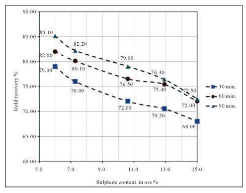
Figure 1. Gold recoveries from high sulphide ores without surfactants.
