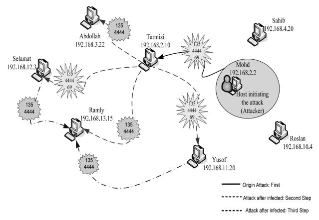
Figure 1. Blaster A incident-Scenario A.
