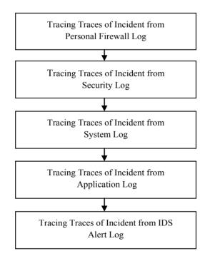
Figure 3. Tracing procedures for tracing evidence of malware incident.
