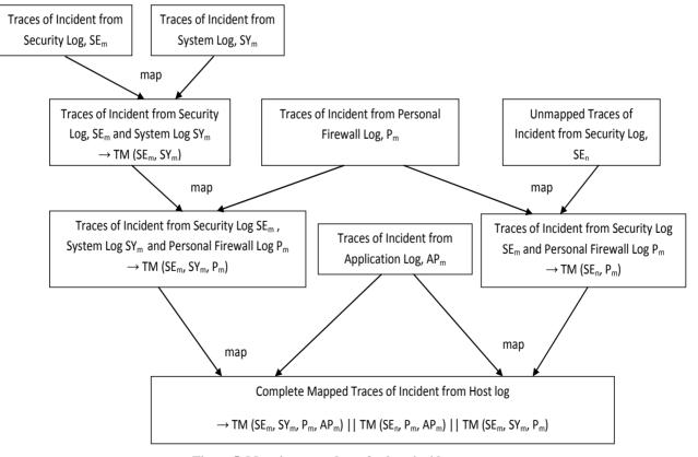
Figure 5. Mapping procedures for host incident traces.
