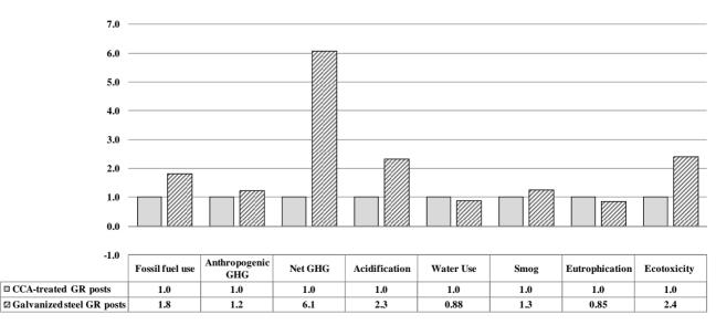
Figure 2. CCA-treated wood and galvanized steel guard rail posts normalized impact comparisons (values normalized to CCA-treated guard rail posts cradle-to-grave = 1.0).
