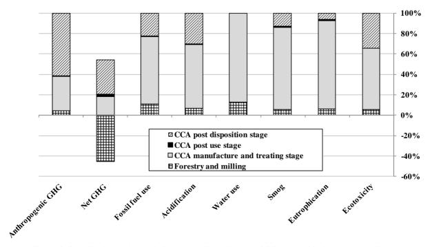
Figure 3. Contributions to impact indicators by life cycle stage of CCA-treated highway guard rail posts.
