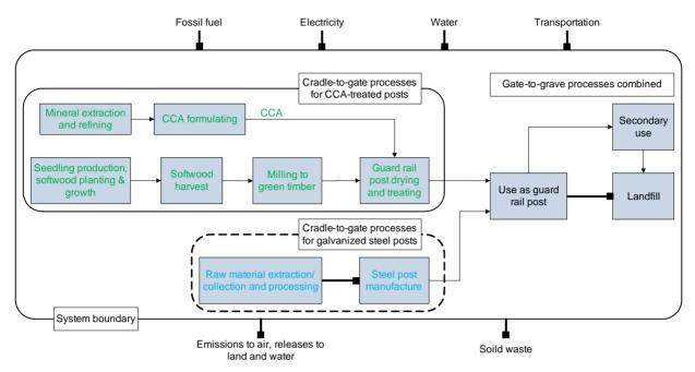
Figure 1. Life cycle stages of CCA-treated guard rail posts.
