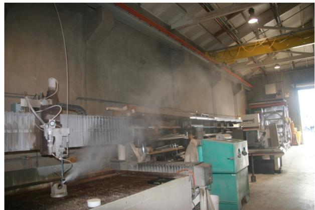
Figure 5. MBARI jet experiment with a 344.7-MPa jet.
