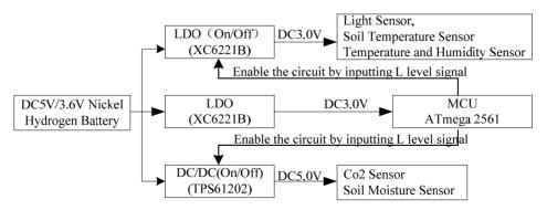
Figure 4. The hardware design of SDEM.
