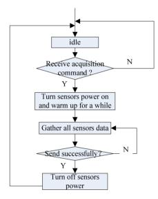
Figure 3. Principle of sensor dynamic energy management.
