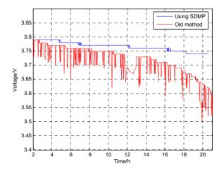
Figure 8. Lift time of sensors between SDEM and before method.
