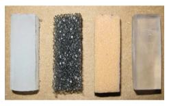
Figure 4. A picture of objects used for grasping: (from left to right) PVC (O<sub>1</sub>), Foam (O<sub>2</sub>), Ethaflex (O<sub>3</sub>) and Plexiglass (O<sub>4</sub>)
