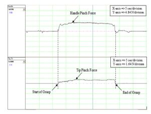
Figure 5. Handle and Tip Pinch Force profile for an object  $(O_3)$  grasped by a subject using palm grasping technique.
