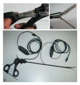
Figure 2. Picture showing (a) Grasper handle attached with strain gauges (b) Grasper tip attached with custom made FSR (c) Sensorized atraumatic fenestrated laparoscopic grasper.
