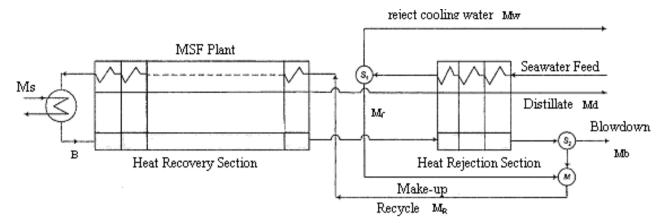
Figure 1. A circulating-brine multistage flash (MSF) desalination plant.
