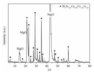
Figure 3. X-Ray diffraction pattern for Bi<sub>1.4</sub>Pb<sub>0.7</sub>Sr<sub>2</sub>Ca<sub>2</sub>Cu<sub>3</sub>O<sub>6</sub>/MgO film prepared following the experimental conditions of sample 5.
