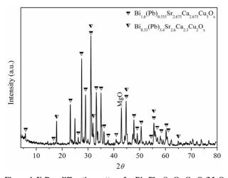
Figure 4. X-Ray diffraction pattern for Bi<sub>1.4</sub>Pb<sub>0.7</sub>Sr<sub>2</sub>Ca<sub>2</sub>Cu<sub>3</sub>O<sub>8</sub>/MgO film prepared following the experimental conditions of sample 9.
