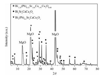
Figure 2. X-Ray diffraction pattern for  $Bi_{1,4}Pb_{1,4}Sr_2Ca_2Cu_3O_{\delta}/MgO$  film prepared following the experimental conditions of sample 7.
