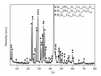
Figure 1. X-Ray diffraction pattern for  $Bi_{1.4}Pb_{1.4}Sr_2Ca_2Cu_3O_{\delta}/MgO$  film, prepared following the experimental conditions of sample 2.
