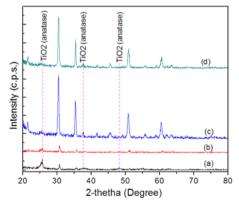
Figure 3. The XRD spectra of TiO<sub>2</sub> thin films using different mass of nano-TiO<sub>2</sub> powder; (a) 1g; (b) 0.4g; (c) 0.1g; (d) 0.05g.
