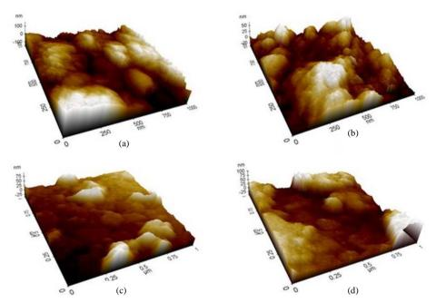
Figure 1. The AFM topography of TiO<sub>2</sub> thin films using different mass of nano-TiO<sub>2</sub> powder; (a) 1g; (b) 0.4g; (c) 0.1g; (d) 0.05g.
