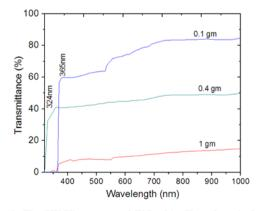
Figure 2. The UV-Vis spectra of  $TiO_2$  thin films deposited using different mass of nano- $TiO_2$  powder.
