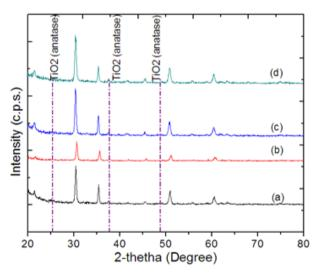
Figure 6. The XRD spectra of TiO<sub>2</sub> thin films using different acetic acid concentration; (a) 0 ml; (b) 3 ml; (c) 10 ml; (d) 30 ml.
