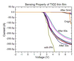
Figure 7. The sensing property of TiO<sub>2</sub> thin film toward IPA solvent.
