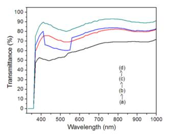
Figure 5. The transmittance spectra of  $TiO_2$  thin films using different acetic acid concentration; (a) 0 ml; (b) 3 ml; (c) 10 ml; (d) 30 ml
