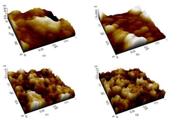
Figure 4. The AFM topography of TiO<sub>2</sub> thin films using different acetic acid concentration; (a) 0 ml; (b) 3 ml; (c) 10 ml; (d) 30 ml.
