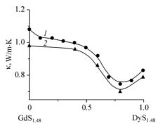
Figure 2. Concentration dependences of thermal conductivity coefficient of solid solutions  $Gd_{1-x}Dy_xS_{1.48}$  at 300 (1) and 400 K (2).
