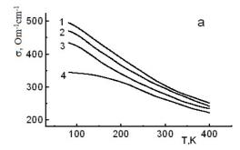
Figure 2. Temperature dependences of electrical conductivity of GdS<sub>1.48</sub> (1), Gd<sub>0.1</sub>Dy<sub>0.9</sub>S<sub>1.48</sub> (2), Gd<sub>0.2</sub>Dy<sub>0.8</sub>S<sub>1.48</sub> (3), Gd<sub>0.3</sub>Dy<sub>0.7</sub>S<sub>1.48</sub> (4).
