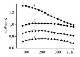
Figure 1. Temperature dependences of thermal conductivity coefficient of  $GdS_{1.48}$  (1),  $Gd_{0.6}$   $Dy_{0.4}$   $S_{1.48}$  (2),  $DyS_{1.48}$  (3),  $Gd_{0.2}$   $Dy_{0.8}$   $S_{1.48}$  (4).
