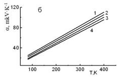
Figure 3. Temperature dependences of Seebeck coefficient of  $Gd_{0.3}Dy_{0.7}S_{1.48}$  (1),  $Gd_{0.2}Dy_{0.8}S_{1.48}$  (2),  $Gd_{0.1}Dy_{0.9}S_{1.48}$  (3),  $GdS_{1.48}$  (4).
