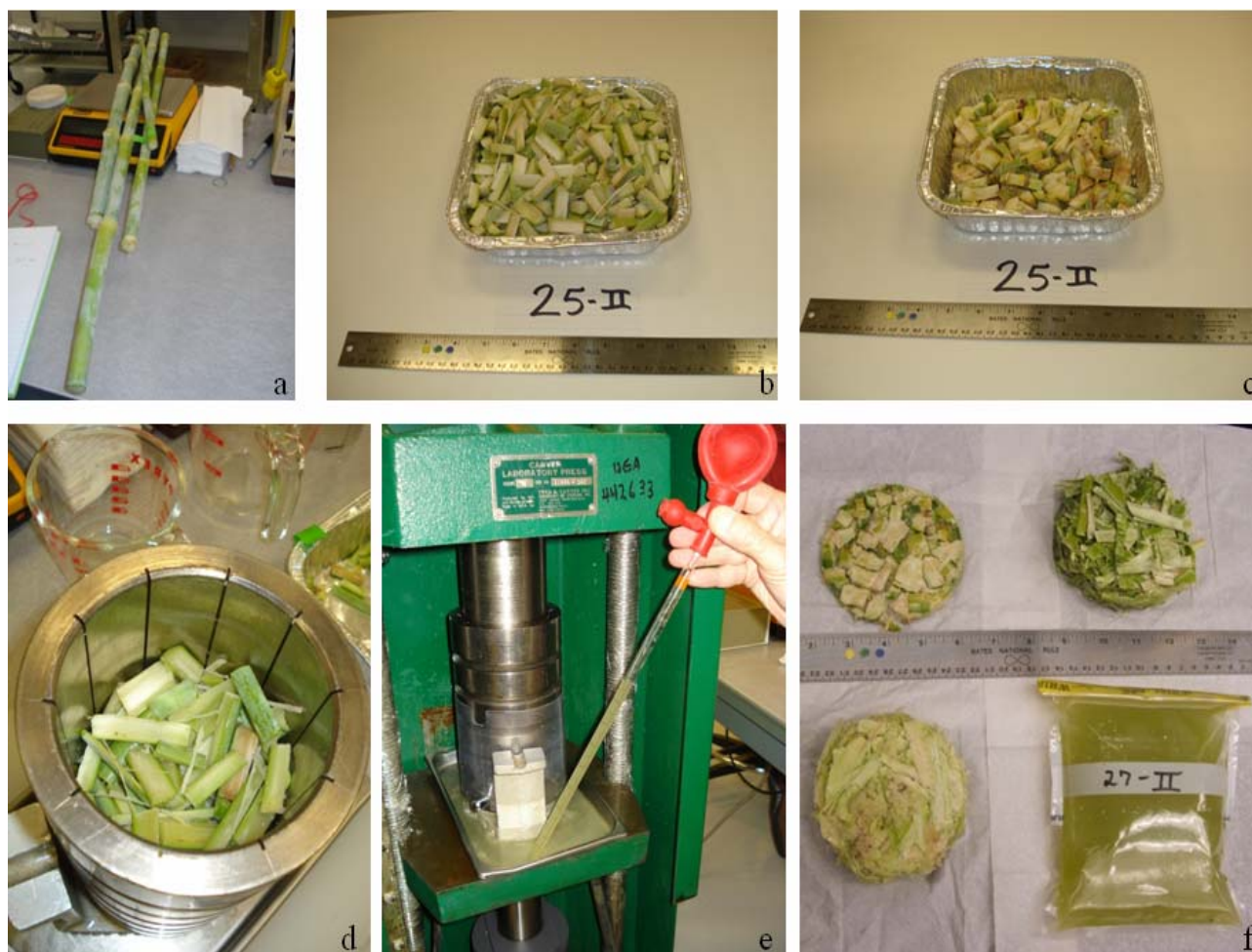
Figure S1. The procedure for collection of stem juice and bagasse from sorghum fresh stems through cutting and pressing.
