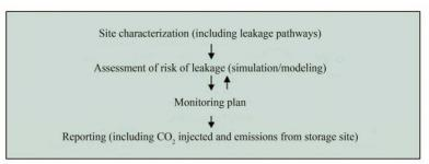
Figure 1. Methodology-estimating, verifying & reporting emissions from CO<sub>2</sub> storage sites; Source: IPCC, 2006.
