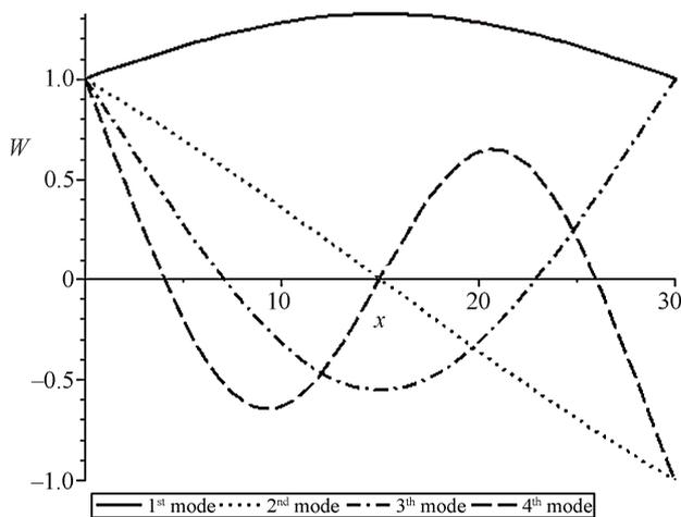
Figure 9. The 1<sup>st</sup> to 4<sup>th</sup> mode shape of  $\text{Al}_2\text{O}_3/\text{Al}$  beams with E-E boundary conditions ( $n = 0.5$ ;  $L/h = 30$ ;  $k_{TR} = 10 \text{ MN/m}$ ;  $k_{RR} = 10 \text{ MN}\cdot\text{m/rad}$ ).
