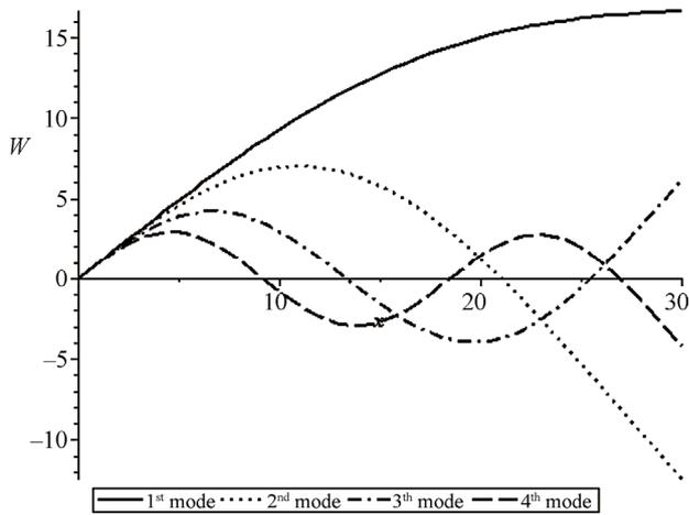
Figure 7. The 1<sup>st</sup> to 4<sup>th</sup> mode shapes of Al<sub>2</sub>O<sub>3</sub>/Al beams with S-E boundary conditions ( $n = 0.5$ ;  $L/h = 30$ ;  $k_{TR} = 10 \text{ MN/m}$ ,  $k_{RR} = 10 \text{ MN}\cdot\text{m/rad}$ ).
