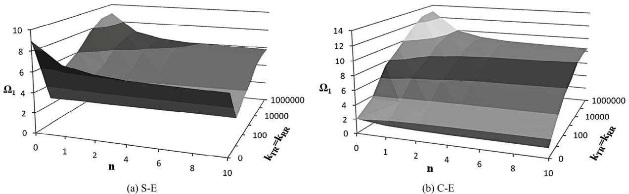
**Figure 6. Fundamental frequency of Al<sub>2</sub>O<sub>3</sub>/Al beams with S-E and C-E boundary conditions ( $L/h = 30$ ).**
