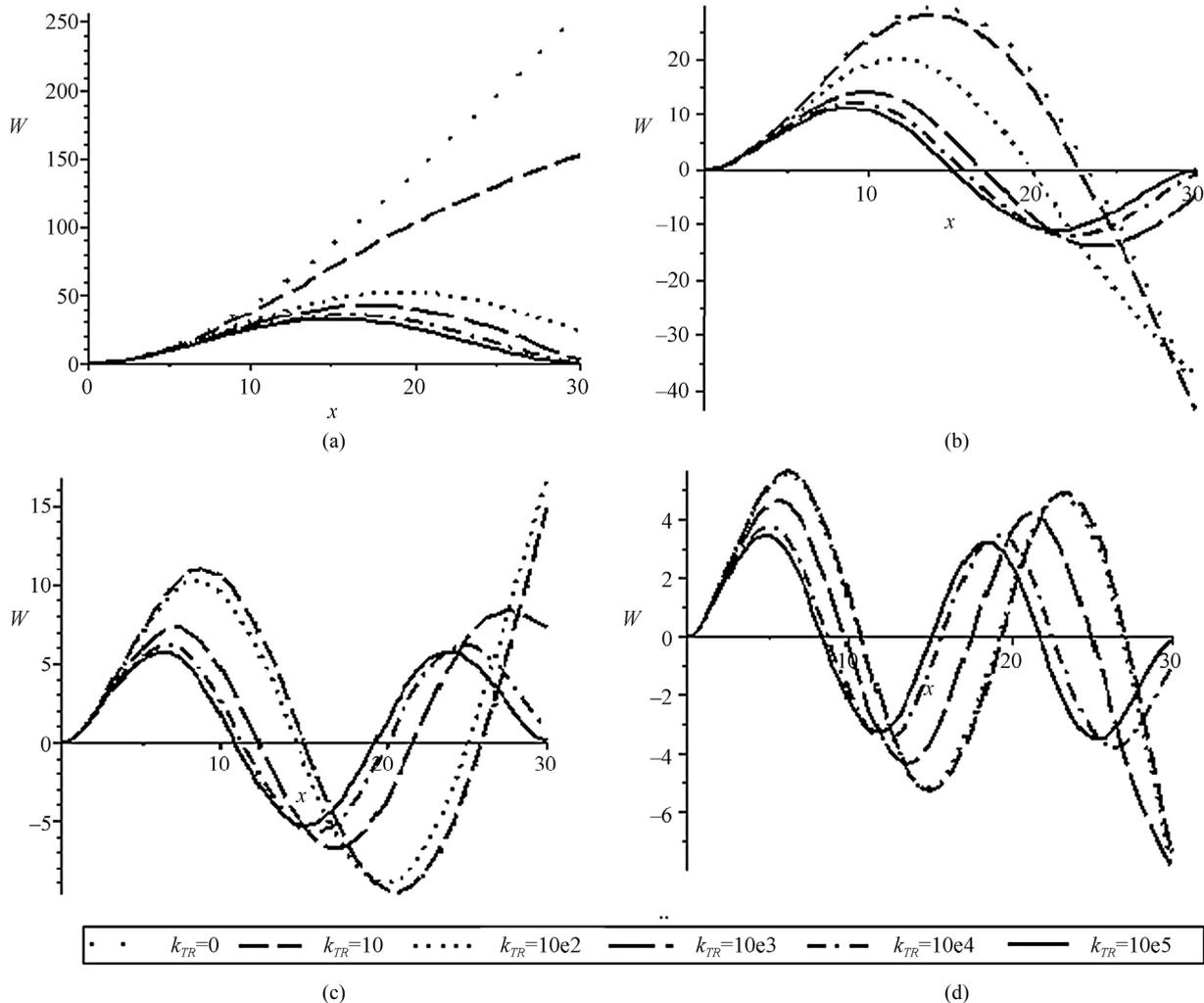
**Figure 5.** The 1<sup>st</sup> to 4<sup>th</sup> mode shapes of  $Al_2O_3/Al$  beams with C-E boundary conditions ( $n = 0.5; L/h = 30; k_{TR} = k_{RR}$ ).
