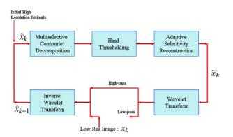
Figure 2. The block diagram of the proposed algorithm for image super-resolution.
