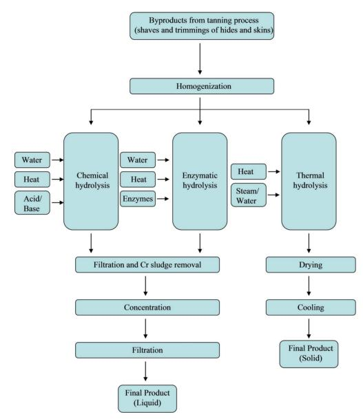
Figure 1. Flow chart of the different productive processes of Cr-containing fertilizers.
