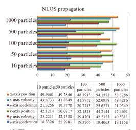
Figure 13. The results, estimation errors versus numbers of particles, using solely particle filtering in a surrounded NLOS propagation environment.
