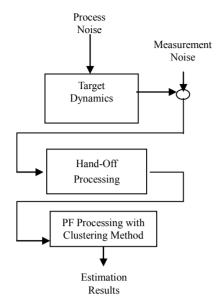
Figure 2. The block diagram of tracking estimation with clustering analysis.
