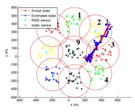
Figure 4. The actual and estimated trajectories of the moving target.
