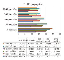
Figure 14. The results, estimation errors versus numbers of particles, using particle filtering with K-means clustering in a surrounded NLOS propagation environment.
