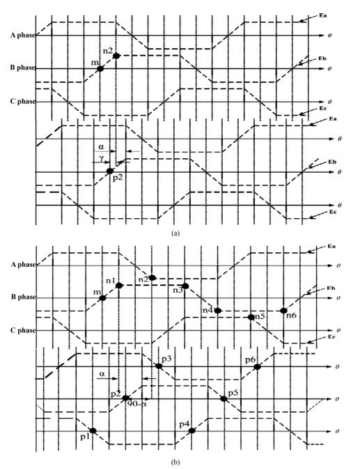
Figure 4. Lagging 90°-α commutation method.
