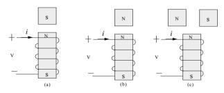
Figure 2. Magnetic fields (a) saturated magnetic field, (b) linear (non-saturated) magnetic field and (c) middle case.
