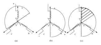
Figure 3. The schematic diagram of initial rotor position detetion. (a) Energized stator winding and rotor position within 180°; (b) Rotor position within 60°.
