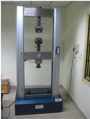
Figure 11. Universal testing machine.
