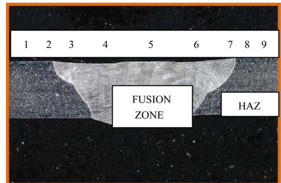
Figure 7. Location of hardness measuring points on the weld joint.
