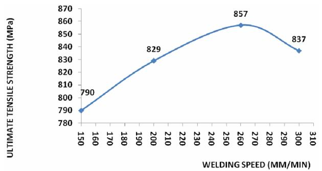
Figure 14. Variation of ultimate tensile strength.
