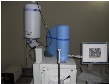
Figure 4. Scanning electron microscope.
