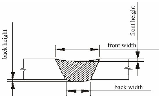
**Figure 1. Typical weld bead geometry.**
