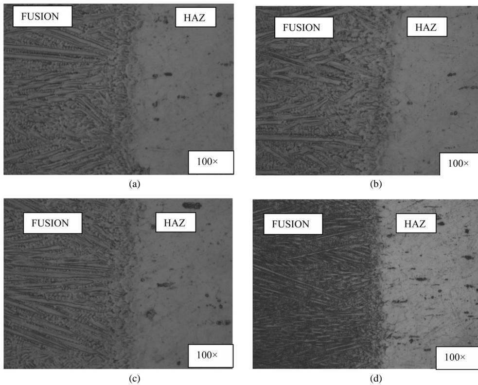
**Figure 3.** (a) welding speed of 150 mm/minute; (b) welding speed of 200 mm/minute; (c) welding speed of 260 mm/minute; (d) welding speed of 300 mm/minute.
