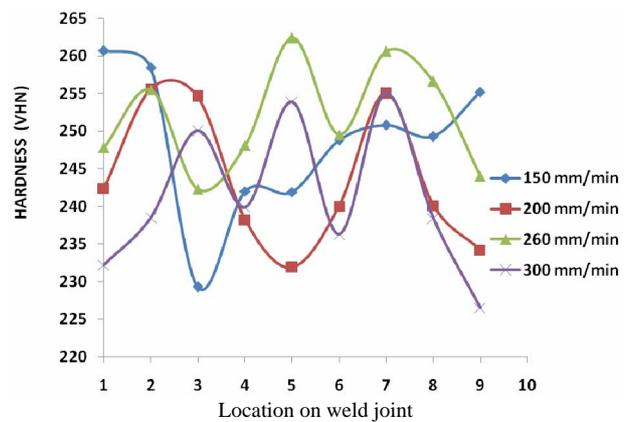
Figure 8. Variation of hardness across the weld.
