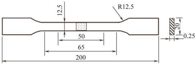
Figure 9. Schematic diagram of tensile specimen as per ASTM E8.
