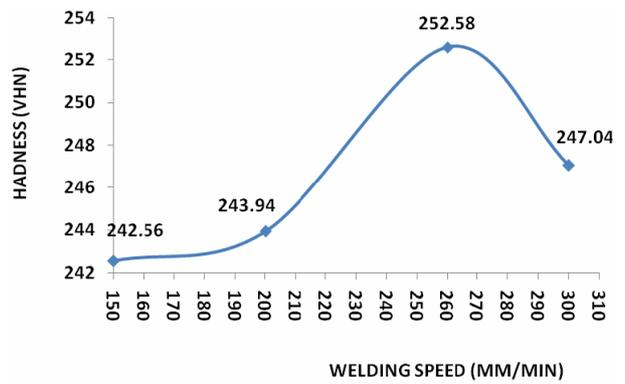
Figure 13. Variation of fusion zone hardness.
