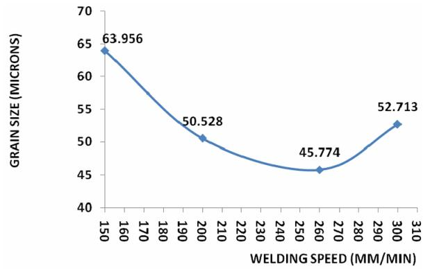
Figure 12. Variation of fusion zone grain size.
