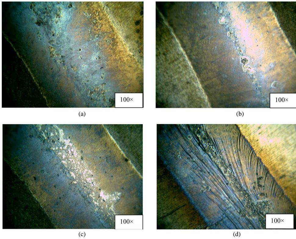
**Figure 2.** (a) welding speed of 150 mm/minute; (b) welding speed of 200 mm/minute; (c) welding speed of 260 mm/minute; (d) welding speed of 300 mm/minute.
