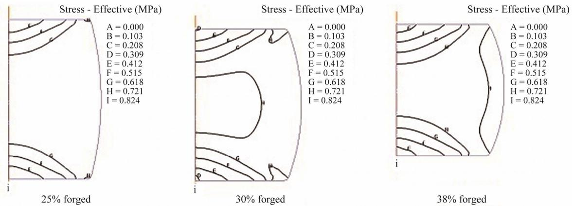
**Figure 8. Simulation results showing effective stress distribution at different stages of compression (5 wt% SiC).**
