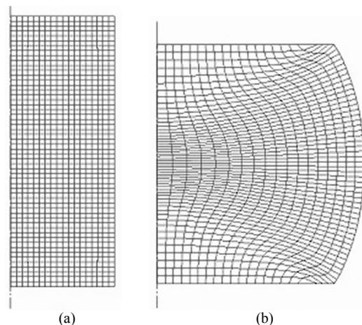
**Figure 5.** FEM – model of the sample (a) before and (b) after compression.
