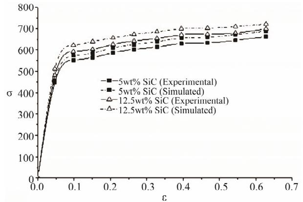
**Figure 7. Variation of  $\sigma$  with  $\epsilon$ . Comparison of experimental and simulated results (5 wt% and 12.5 wt% of SiC).**
