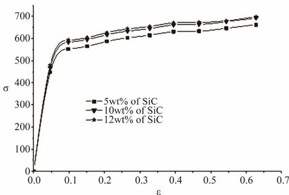
**Figure 4.** Variation of equatorial stress with height strain.
