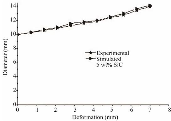
**Figure 6. Variation of equatorial diameter with height reduction. Comparison of results from experiment and simulation (5 wt% SiC).**
