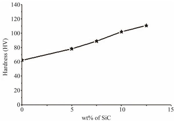
**Figure 3.** Variation of hardness with weight percentage of SiC.
