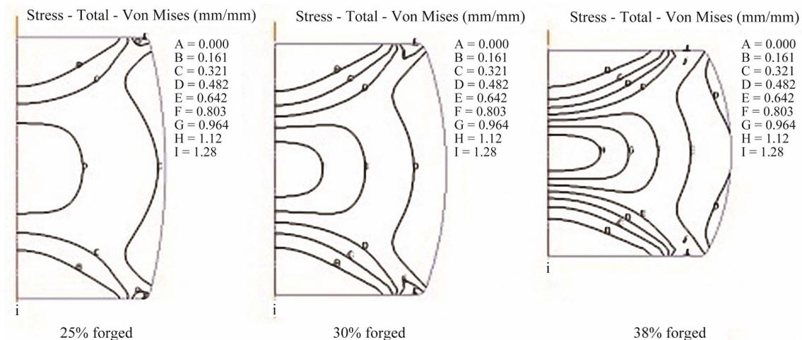
**Figure 9. Simulation results showing distribution of Von-mises strain at different stages of compression (5 wt% SiC).**
