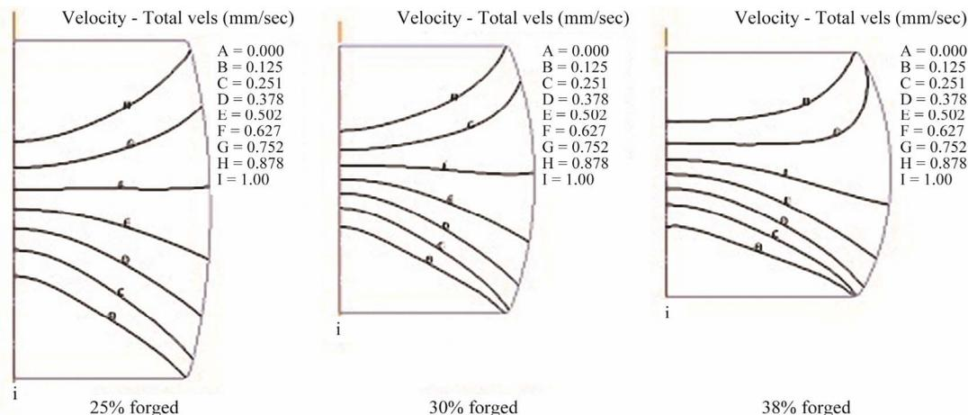
**Figure 10. Simulation results showing variation in velocity within the specimen at different stages of compression (5 wt% SiC).**
