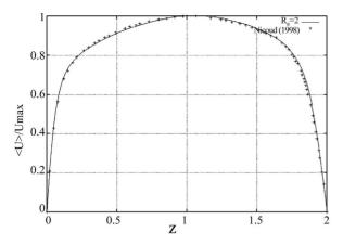
Figure 5. Mean Stream-wise velocity profile normalized with maximum velocity for the entire channel.
