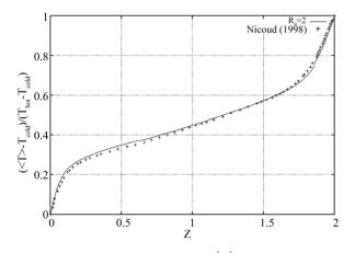
Figure 6. Mean Temperature for  $\frac{\langle T \rangle - T_c}{\Delta T}$  for the entire channel along wall normal direction, for  $R_{\theta} = 2$ .
