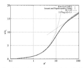
Figure 3. Mean velocity profile in log units for R = 1.01 with  $u^+ = z^+$  and  $u^+ = 2.5 \ln z^+ + 5.5$ .
