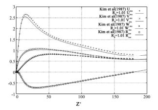
Figure 4. Variation of turbulent stresses  $(\langle u'^2 \rangle, \langle v'^2 \rangle, \langle w'^2 \rangle, \langle u'w' \rangle)$  along normal direction  $(z^+)$  for  $R_{\theta} = 1.01$ .
