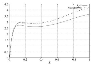
Figure 8. Variation of  $T_{rms}$  along the wall normal direction  $(z^+)$  for  $R_{\theta} = 2$ .
