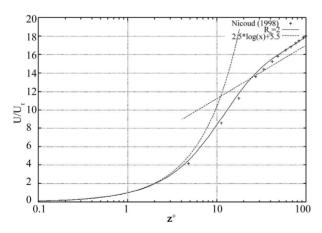
Figure 7. Mean velocity profile in log units along the channel for  $R_{\theta} = 2$ .
