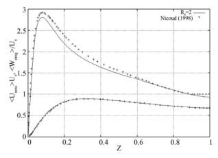
Figure 9. Variation of RMS velocities along the wall normal direction (z) for  $R_{\theta} = 2$ .
