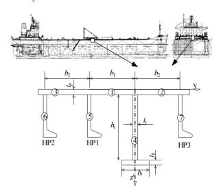
Figure 1. Location and configuration of the investigated panel of the tanker deck.
