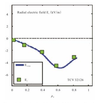
Figure 3. Example of radial electric field  $E_r(r)$  profile calculation in a typical ohmic discharge in TCV tokamak [36].  $\rho_{\Psi}$  is the effective radius of the tokamak magnetic surface. Solid curve is the experimental  $E_r(r)$  profile; squares are the  $E_r(r)$  values calculated with Equation (11) using the experimental toroidal rotation plasma velocity profile.
