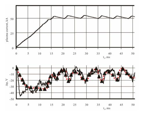
Figure 2. Time dependence of plasma current  $I_p(t)$  and the tokamak chamber electric potential  $\Delta \varphi(t)$  during the discharge, T-11M tokamak [23]. Solid curve is the experimental dependence of  $\Delta \varphi(t)$ ; triangles and dashed curve are the theoretical dependence.
