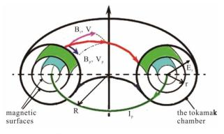
Figure 1. A sketch of tokamak.
