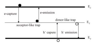
Figure 1. Energy band diagram for a semiconductor with deep-level traps.  $E_C$  is lower edge of the conduction band while  $E_V$  is the upper edge of the valence band.
